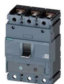
circuit breaker 3VA1 IEC frame 250 breaking capacity class S Icu=36kA @ 415V 3-pole, line protection TM240, ATAM, In=250A overload protection Ir=175A...250A short-circuit protection Ii=5...10 x In nut keeper kit
